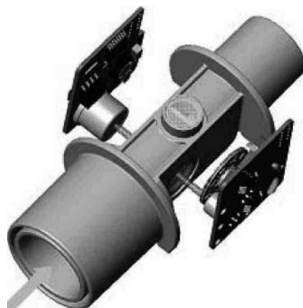
Figure 4. MASIMO SWEDEN AB IRMA IR light path through the IRMA airway adapter.
